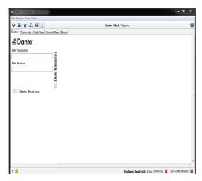
The matrix is divided into transmitter and receiver two parts. The devices (two or more) connected to the same routing appear both in the transmitter and receiver end, you can select the signal sending through the matrix.
